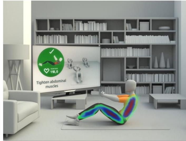
The sensor system integrated in smart textiles like body fitting yoga and athletic wear, enables the monitoring of movements through the measurement of pressure, muscle contractions, and further parameters. The user can retrieve analyses and tips on his smartwatch or screen in real time, to evaluate and optimize his activities.
